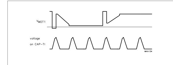
If the chosen value of CAP-TI is too small oscillations can occur in certain positions of a blocked rotor. If the chosen value is too large, then it is possible that the motor may run in the reverse direction (synchronously with little torque).
